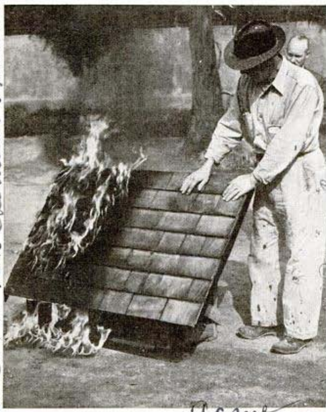
Flames still lick across untreated shingles long after gasoline has been burned from the fireproofed portion leaving it cool
